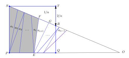
To end with a vertical segment, the product of the ratios of "+" and "-" should equal  $\overline{RO}/\overline{SO}$  and  $\overline{QO}/\overline{PO}$ :
